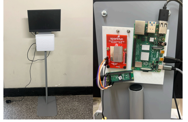
Fig. 2 Left: Ambulation station setup with external antenna on stand. Right: Hardware setup with M7E Hecto RFID reader, Raspberry Pi 5, and Pico microcontroller bridged to the Pi
